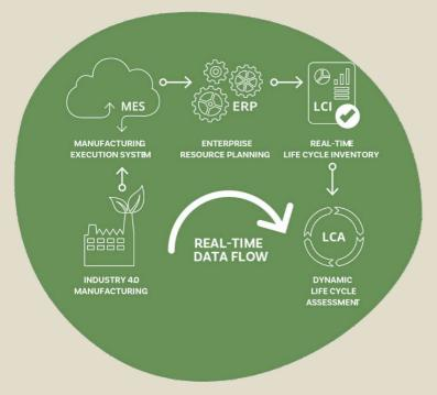
This sensor network is connected to the Manufacturing Execution System (MES), a software solution that links the factory environment to the Enterprise Resource Planning (ERP) management system. This connection enables the acquisition of real-time process data, useful not only for operations management but also for inventory analysis for Dynamic Life Cycle Assessment (LCA).
